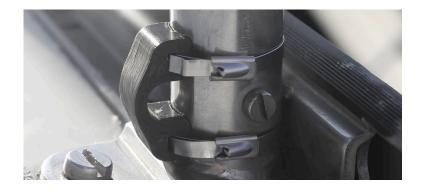
Cut off excess cable tie and thread ends into fitting to avoid injury.
