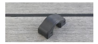
3D printed stanchion fitting made with ABS filament.
