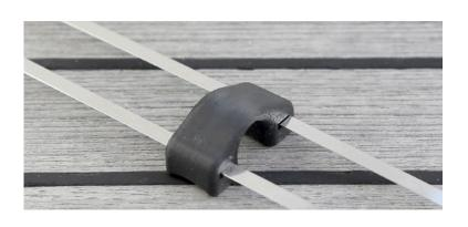
Standard 5mm wide stainless steel cable ties are threaded into the cut outs of the fitting. When tightening the cable ties, push back the locking ball with a small flat-head screw driver to achieve a tight fit.
